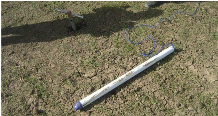
Fig. 5.2.5b Volumetric moisture probe waiting to be installed
