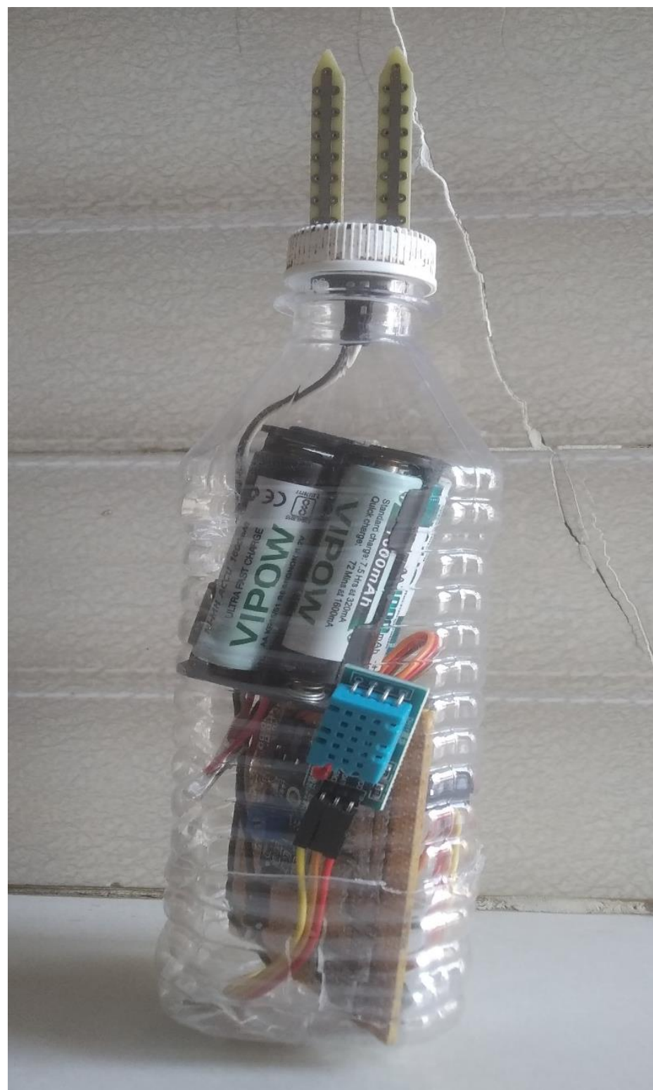
Fig.13.8a prototype of IoT module
