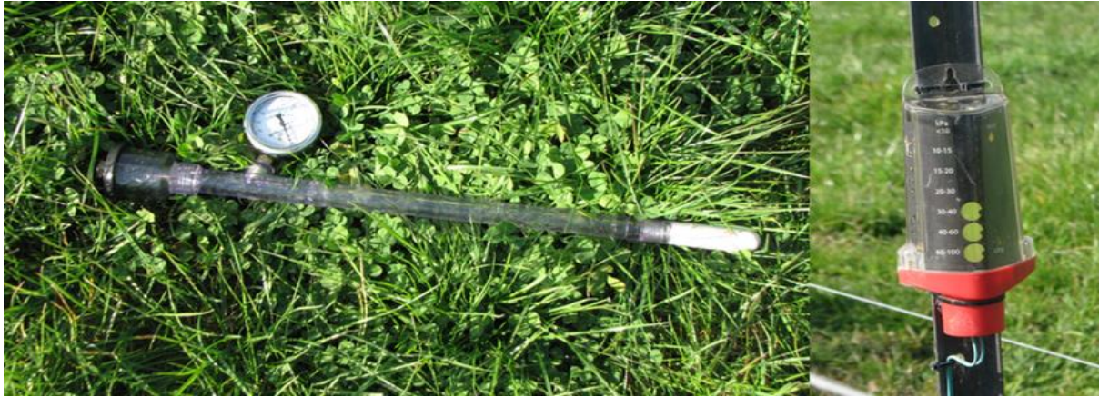
Fig. 5.2.5a Tensiometer uninstalled (left), GDot (right)
